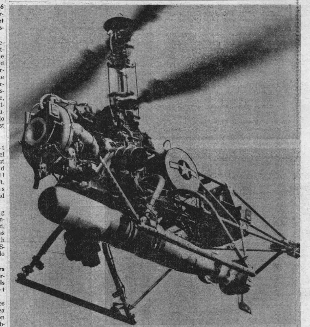
A DRONE HELICOPTER carries the Mark 46 during test operation off Long Beach. The new weapon is capable of hunting, overtaking and killing today's modern conventional and nuclear submarines. NOTS Pasadena program's technical development director.
