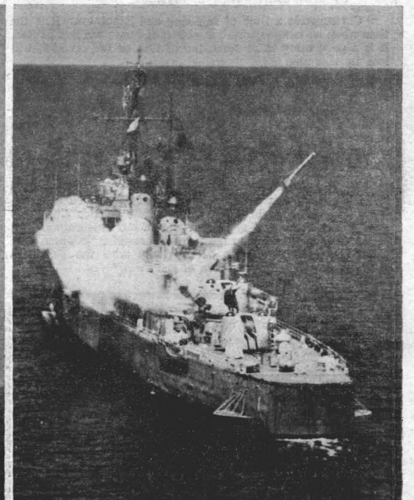
ANOTHER WAY to launch the Mark 46 torpedo is with ASROC, another NOTS "first." Here's a shot from destroyer.
