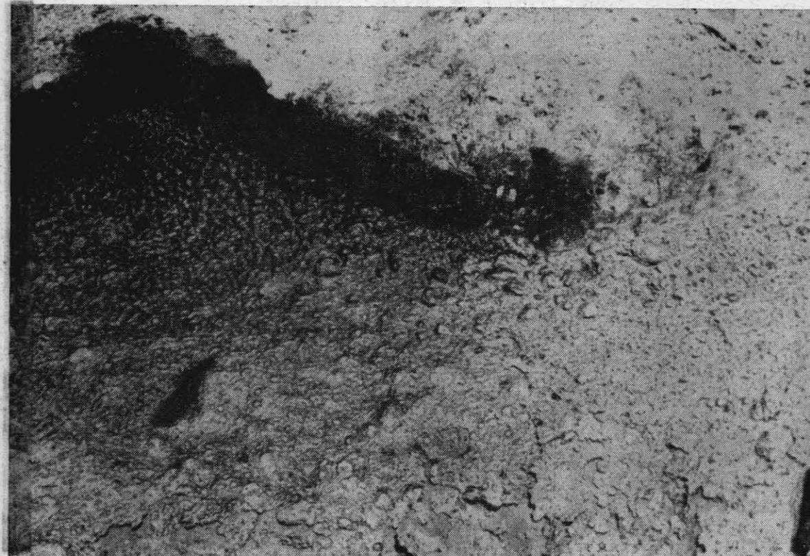
DESERT SAND was solidified into glass by intense heat of burning propellant.
