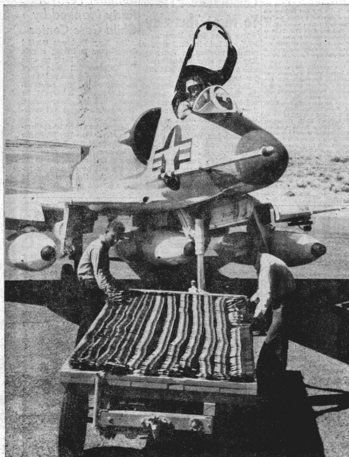
HIGHPEG, the Navy's fastest gun, is shown with its 887 armor-piercing 20mm cannon shells, which gives the Skyhawk fighter 10 times the gun firepower of its World War II predecessor. Gun underwent tests here and was demonstrated during President Kennedy's visit to NOTS in June of '63.
