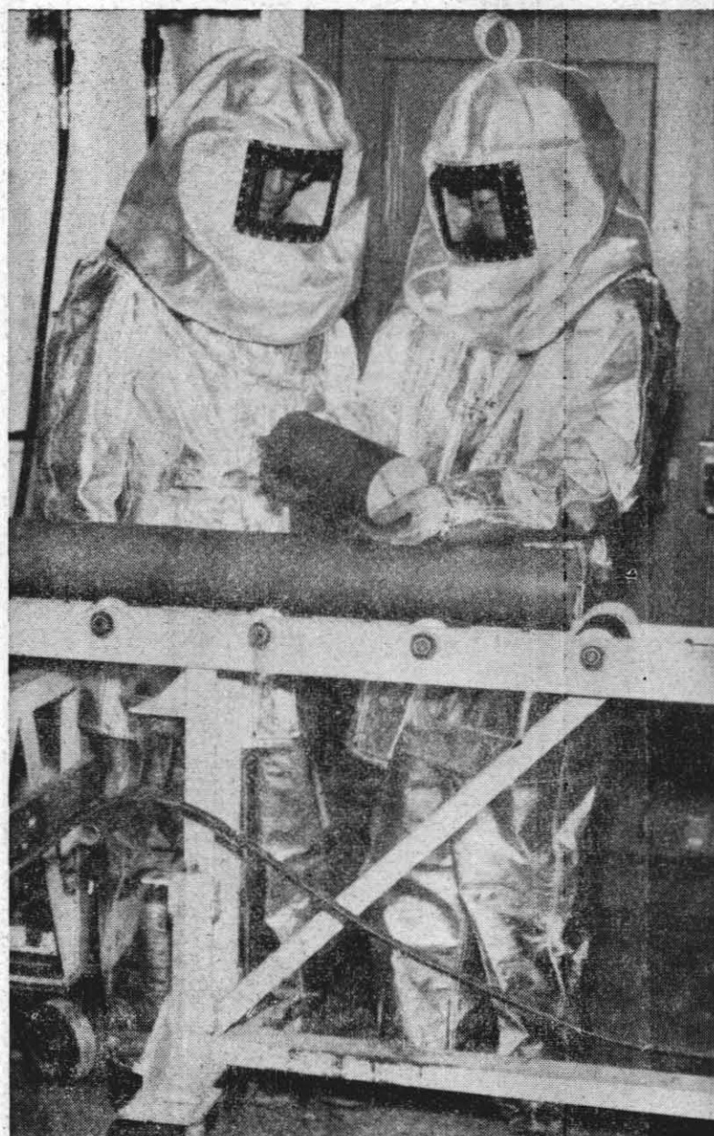
RAP, Rocket Assisted Projectile's fluorocarbon propellant is examined by Charley Rodgers and Jud Eldridge of the Propulsion Development Department. Project incorporates use of a rocket motor to give 5-inch projectile longer range. Men wear protective clothing. Both are pioneers in solid propellant research at NOTS.
