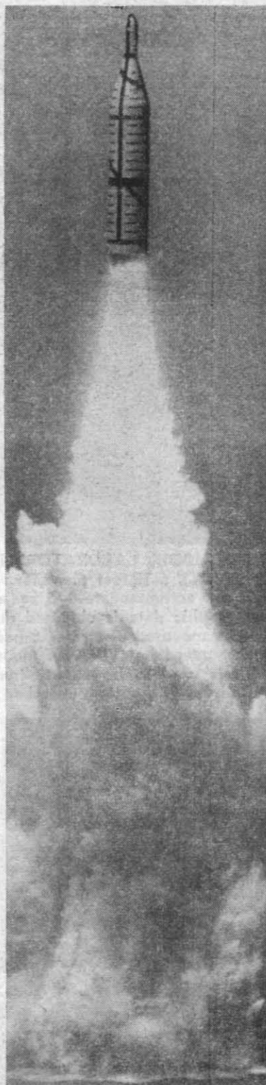
POLARIS — Launched from underwater, Polaris makes a short controlled flight at the San Clemente Island sea range. These tests demonstrated the ability of Polaris to accomplish the transition from underwater launch to controlled powered flight — a forward step in the development of the Navy Polaris Missile prior to operational service aboard nuclear powered submarines.
