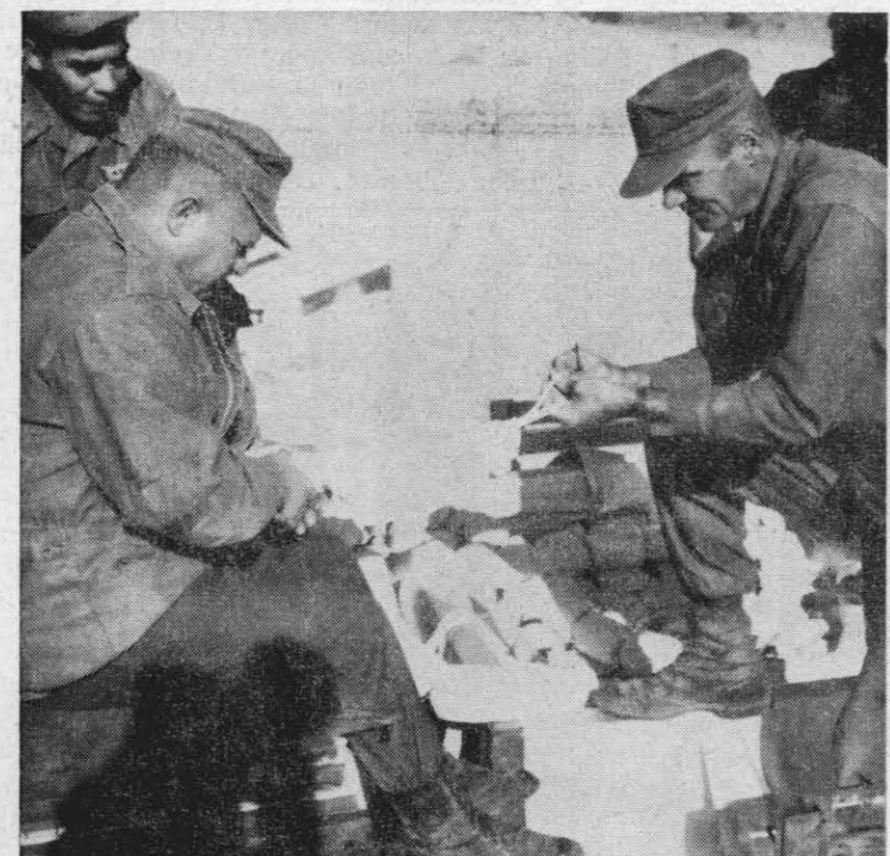
FUSE IS ATTACHED to Line Charge after charge has been carefully placed in layers so line won't foul when payed out as towing rocket is fired down range.
