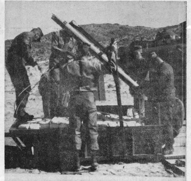
MARINES FASTEN towline of Line Charge to NOTS-developed 5-inch rocket. Rocket will tow charge down range. Charge can be used to clear land mine fields.
