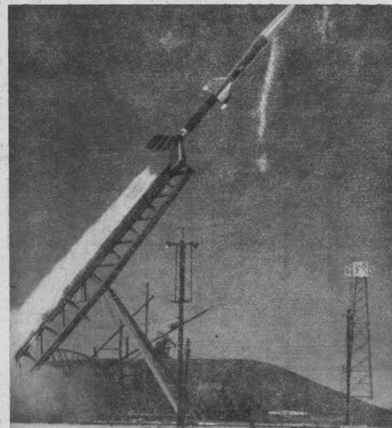
'BIG STOOP,' a two-stage surface-to-surface rocket, forerunner of today's Army's one-stage 'Honest John,' is fired from the Vantos I launcher on the old G-1 Range during 1950.
