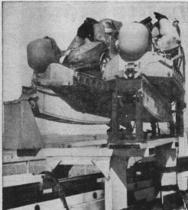
TWIN DUMMIES, nicknamed Castor and Pollux after the bright stars in the Gemini constellation, lie strapped in mock pilot seats for one of the ejection tests now under way at NOTS. They're atop 150-foot tower in Randsburg Wash.
