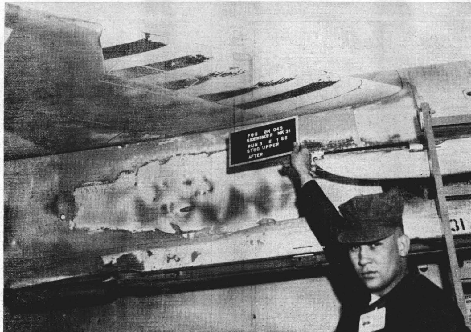
F8U-2N PROTECTION—Silicone coating on the F8U-2N Crusader is still intact but thin after three firings. The coating was developed to protect craft against the erosive gases of air-launched missiles. Elder Bartel of the Plastics Section,
