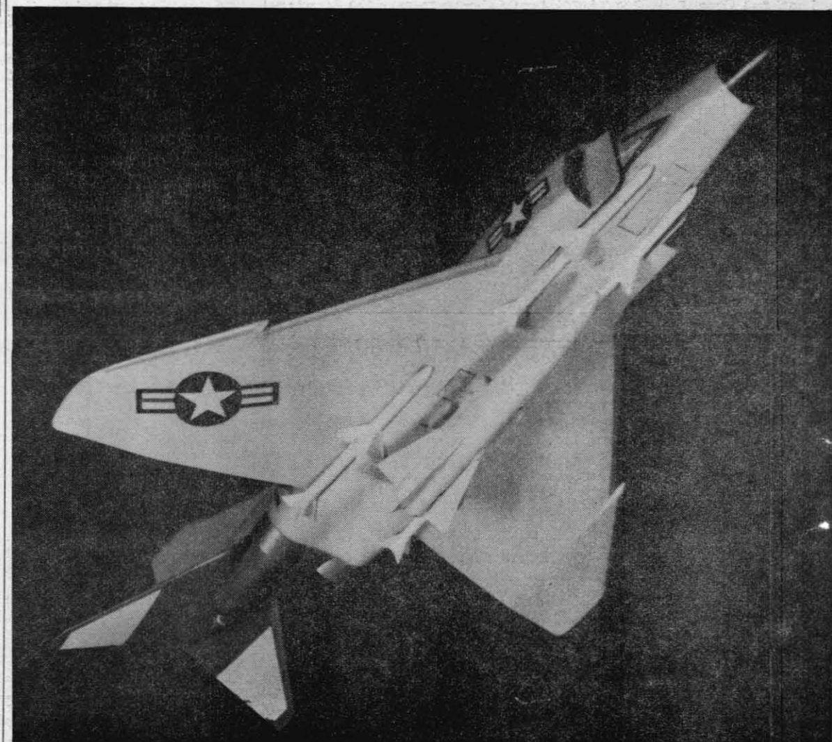
CALEB —Under the fuselage of a McDonnell F4H Phantom II fighter model, Sparrow air-to-air missiles flank the NOTS-designed and developed Caleb which can be launched from any point in the world that is accessible to the Navy's aircraft.
