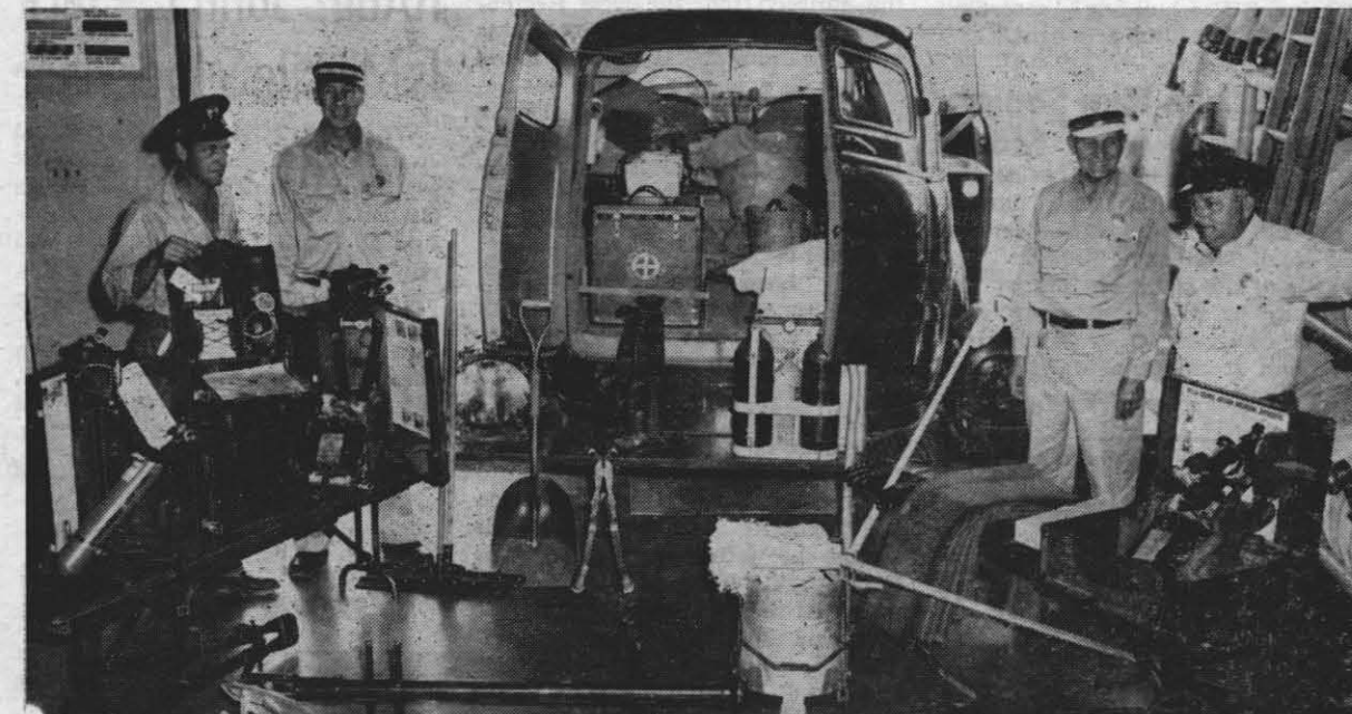
RESCUE TRUCK EQUIPMENT is checked daily to insure that everything is operating properly and is in good repair. Each driver, when he is assigned to the vehicle for a shift must make this check and report that the truck is "in service" and ready. Inspection of the
