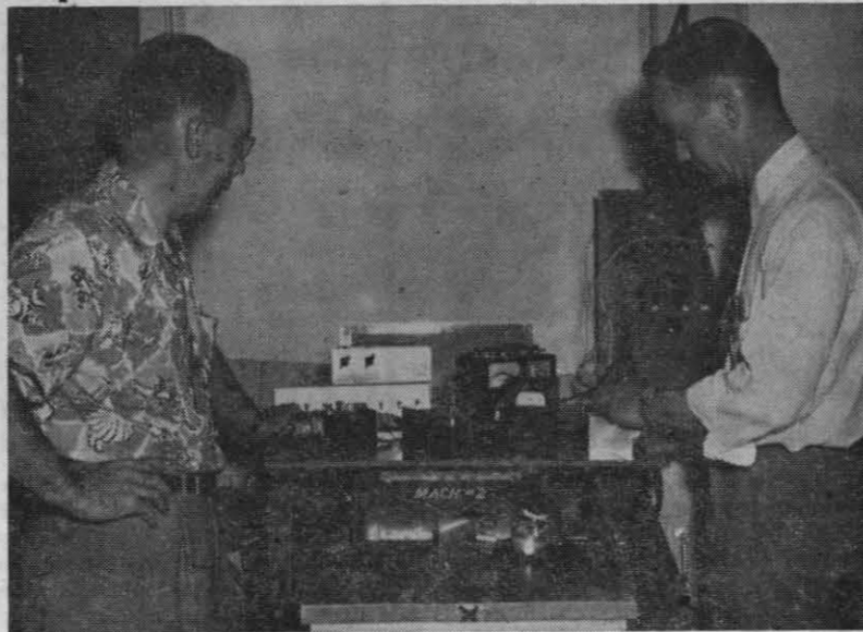
DR. VICTOR B. COREY, right, technical director of the Donner Scientific Instrument Company, demonstrates one of his company's first production servo accelerometers to Paul Driver, who developed the original models at NOTS. The unit, with the electro-mechanical element removed from its case, can be seen in the foreground resting on a mechanical shake table.
